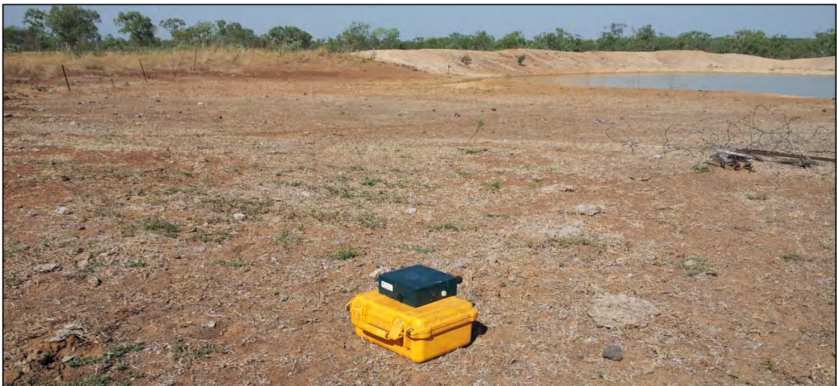
Figure 2.3 – SM2Bat device set up in study area
